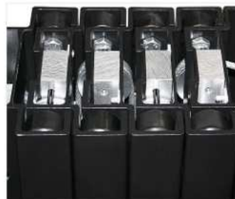
Cable resend system with steel pulleys.
