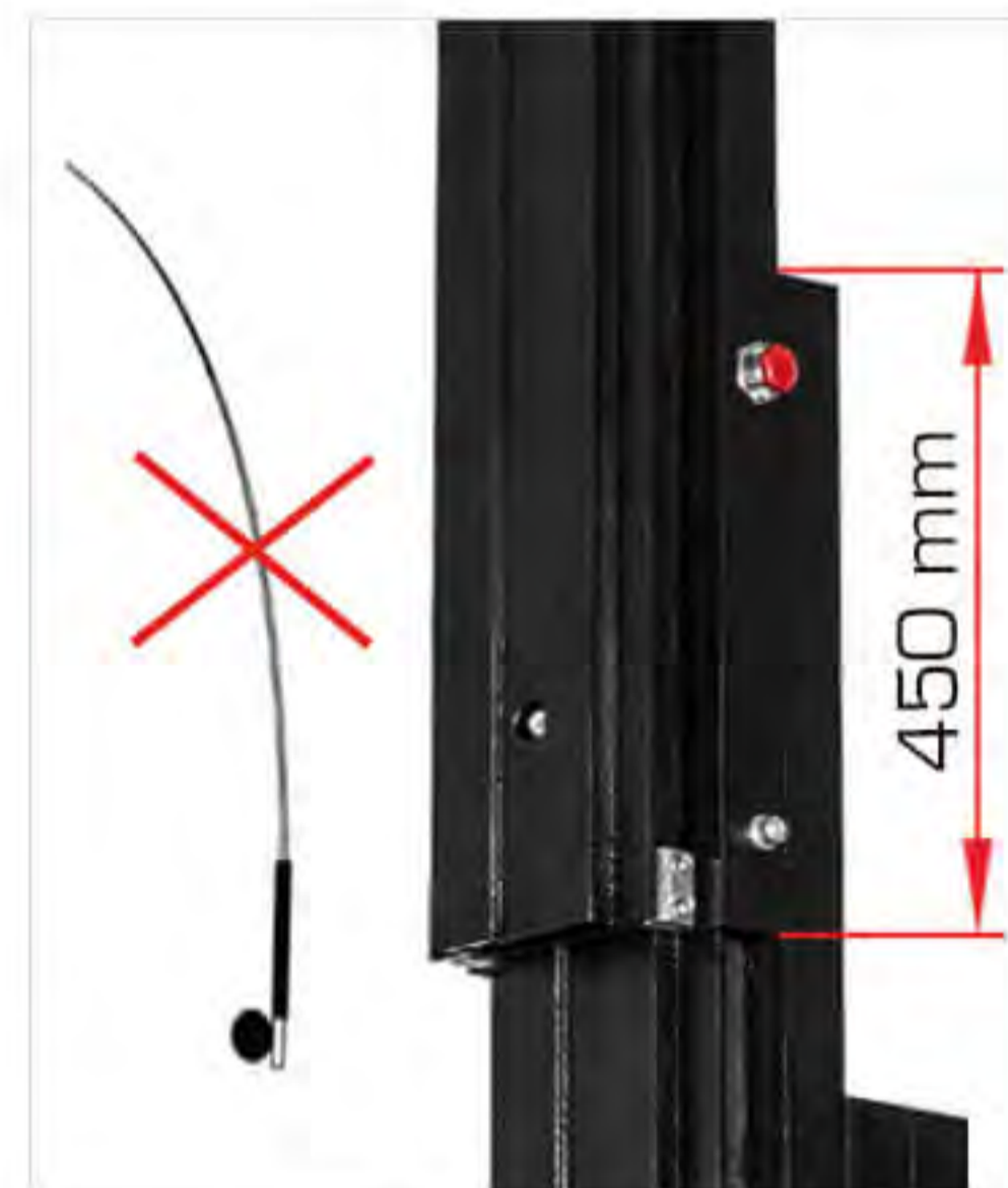
More mast overlap. Prevent fishing rod effect.
