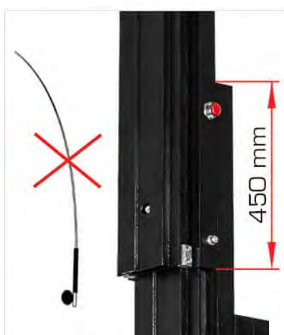
More mast overlap. Prevent fishing rod effect.
