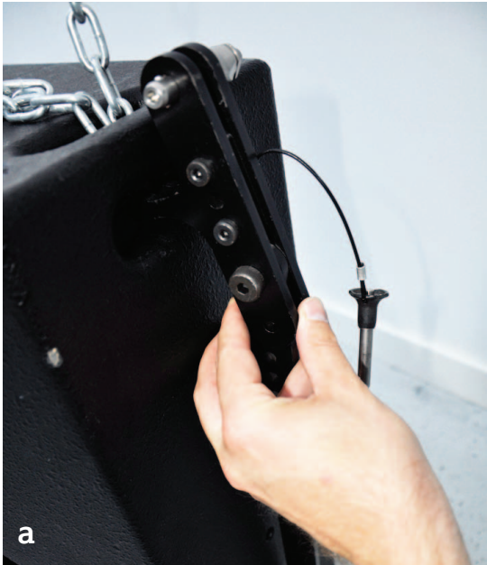
Open the pin to tilt the top part of the BBT24 to attach it to the upper handle.
