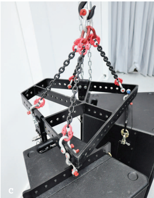
Attach the ASK44 to the MCT24 using the shakles delivered with the ASK44 . The main cradle should always hang almost straight.
