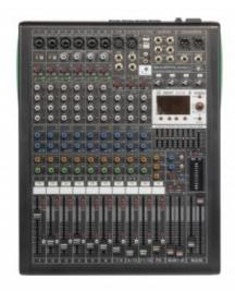
Compact analog mixer with 32-bit DSP and full duplex audio interface, 99 effects, Bluetooth connectivity, and multimedia player. 4 independently selectable auxiliary output groups with matrix selector. 9-band equalizer on master. +48V phantom power
