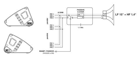
Figure 3.2 - Wiring diagram
